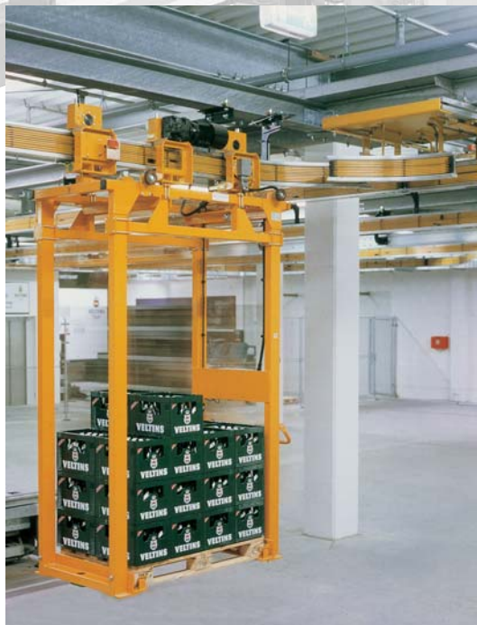
Electric overhead monorail with conductor rail - trolley on the way to the high bay storage
